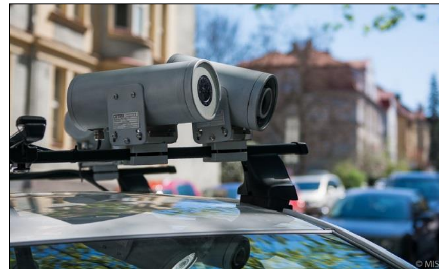
Cameras of the roof of the monitoring car ↳ InfraRed for scanning the number plates → Visible spectrum camera for overview
